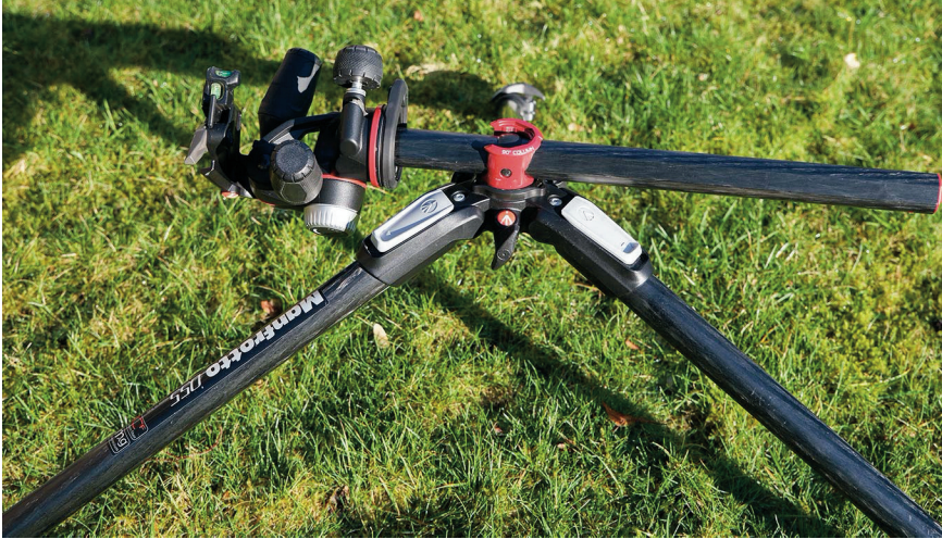
Tripod legs spread to position the camera nearer to the ground
