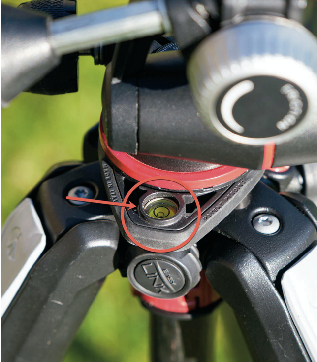
Spirit level on the tripod legs to ensure they are level
